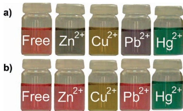
Figure 2. Changes in the color of receptor 4 , in (a) \text{CH}_3\text{CN} and (b) \text{CH}_3\text{CN}/\text{H}_2\text{O} 3/7, upon addition of the corresponding cation.
